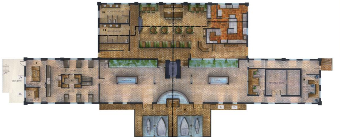
Figure 1: Lower level of the renovated lodge showing berths for boats , a reception and display area, as well as a laboratory on the left side of the plan Watermark student design team
