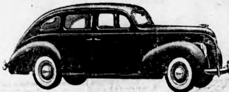
DE LUXE FORD V-8 . . . 112" wheelbase; 85-hp. engine; Improved Easy-Action Safety Brakes; Mohair or Broadcloth upholstery; Twin horns, tail lights, sun visors; Clock; 6.00" tires, white side-walls are extra; 8 body types; 6 colors.
