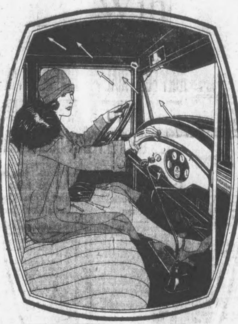
This diagram shows how the Studebaker no-draft ventilating windshield, when opened outward, directs the air up over the occupants' heads. The convenient handle on the dash adjusts the windshield to any desired position. A hidden trough under the cowl carries off rain when the windshield is set for storm-proof ventilation.
