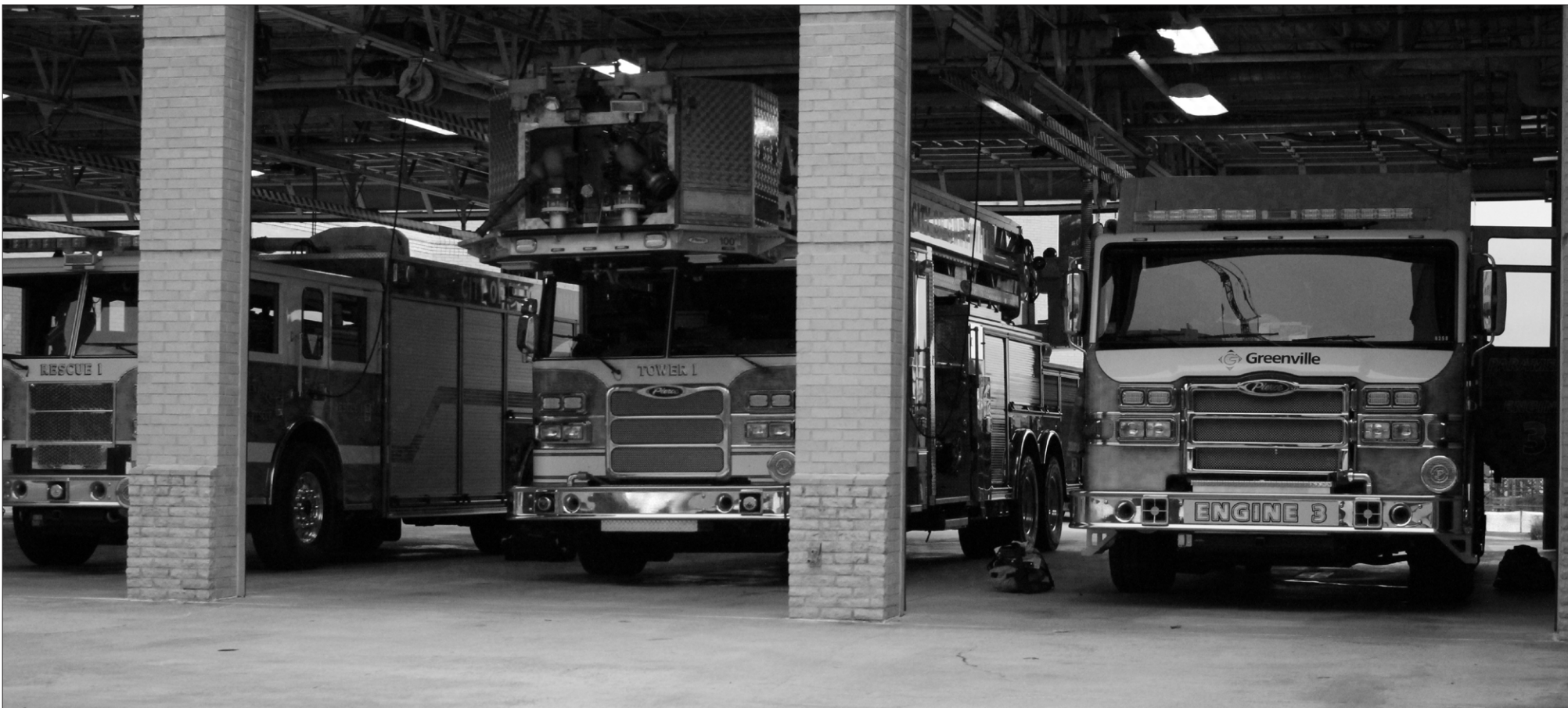
Engine 3, Tower 1 and Rescue 1 sit in the engine bay at Greenville Fire/Rescue Station 1 Tuesday evening. Tower 1 is a 100-foot ladder truck tasked with saving individuals from high-rise buildings.
