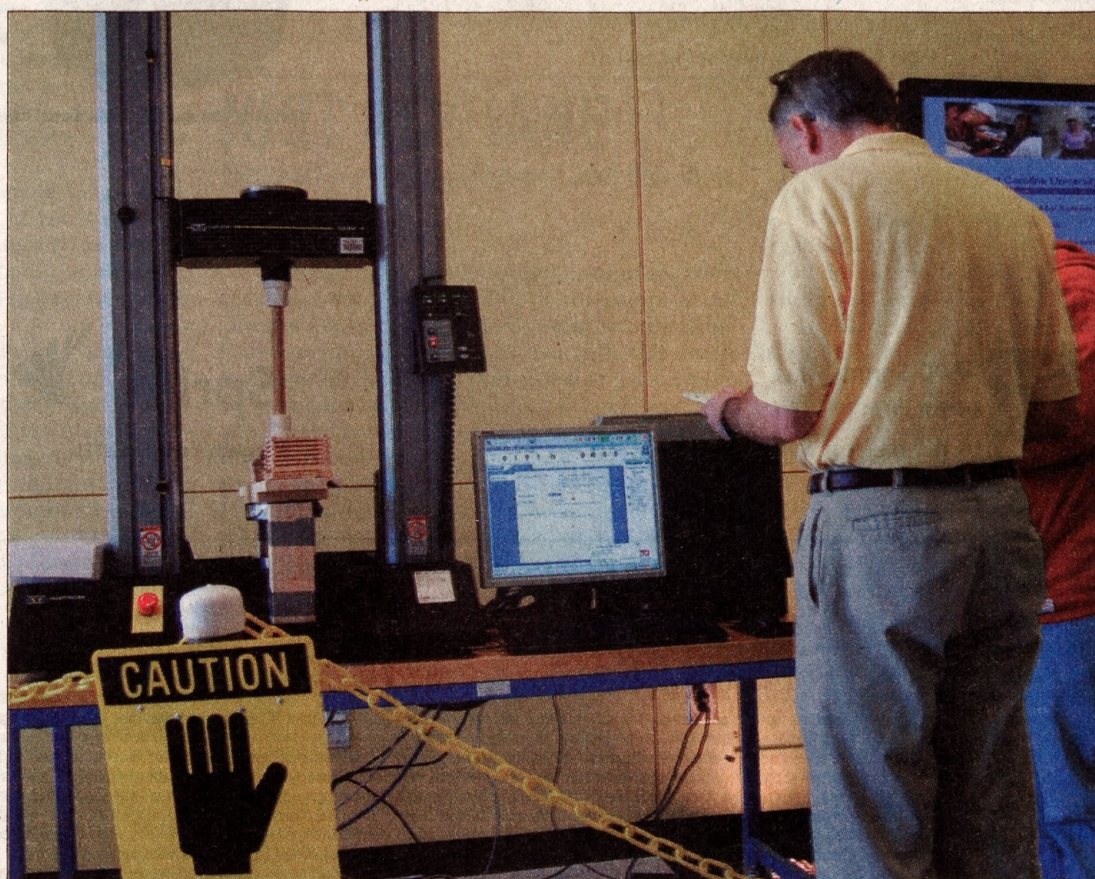
A contestant's bridge is tested for strength and durability during Engineering and Technology Day.
