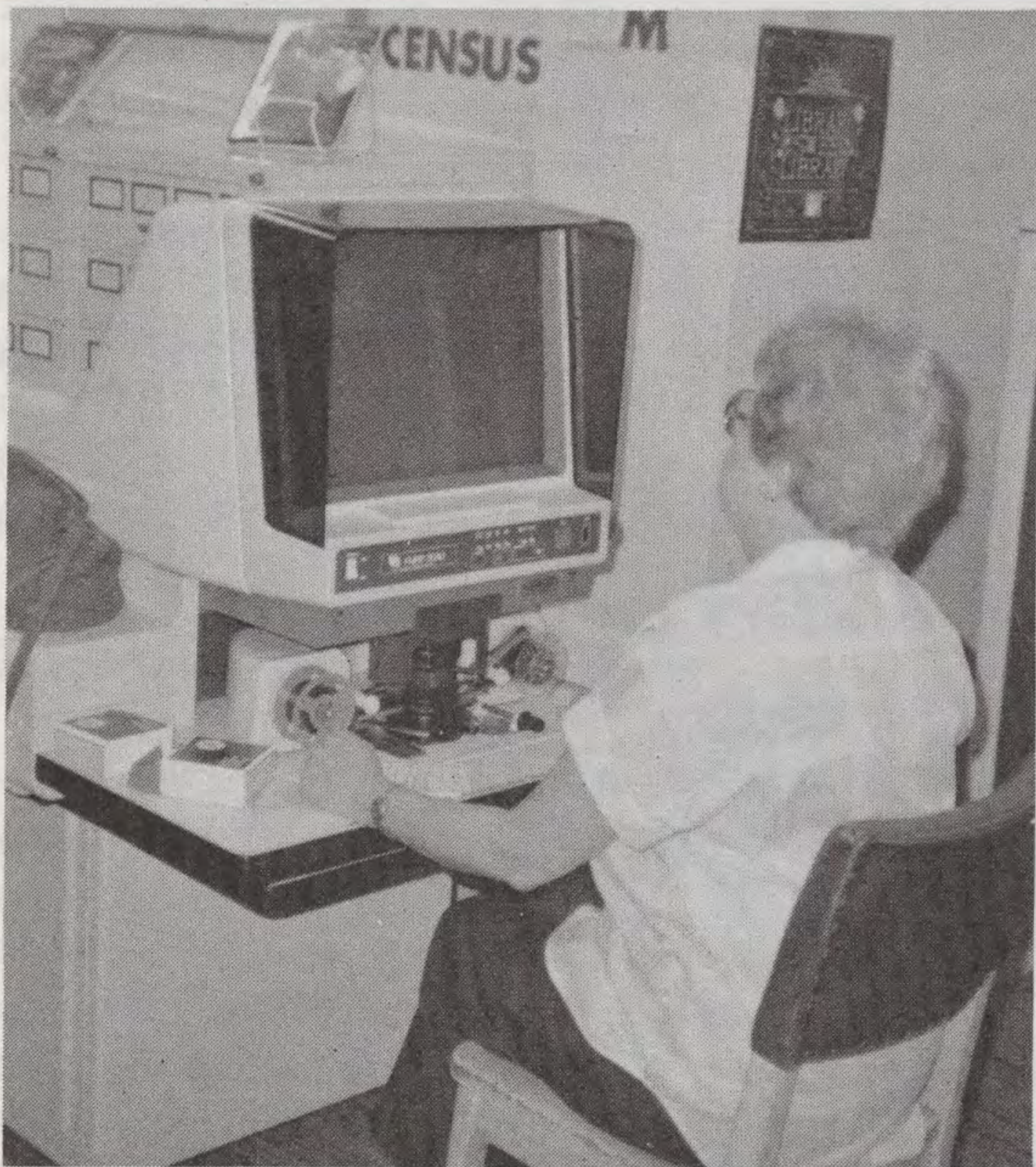
A microfilm reader/printer is a virtually essential piece of equipment in local history collections with microfilm holdings. Photograph courtesy of Forsyth County Public Library, Winston-Salem.
