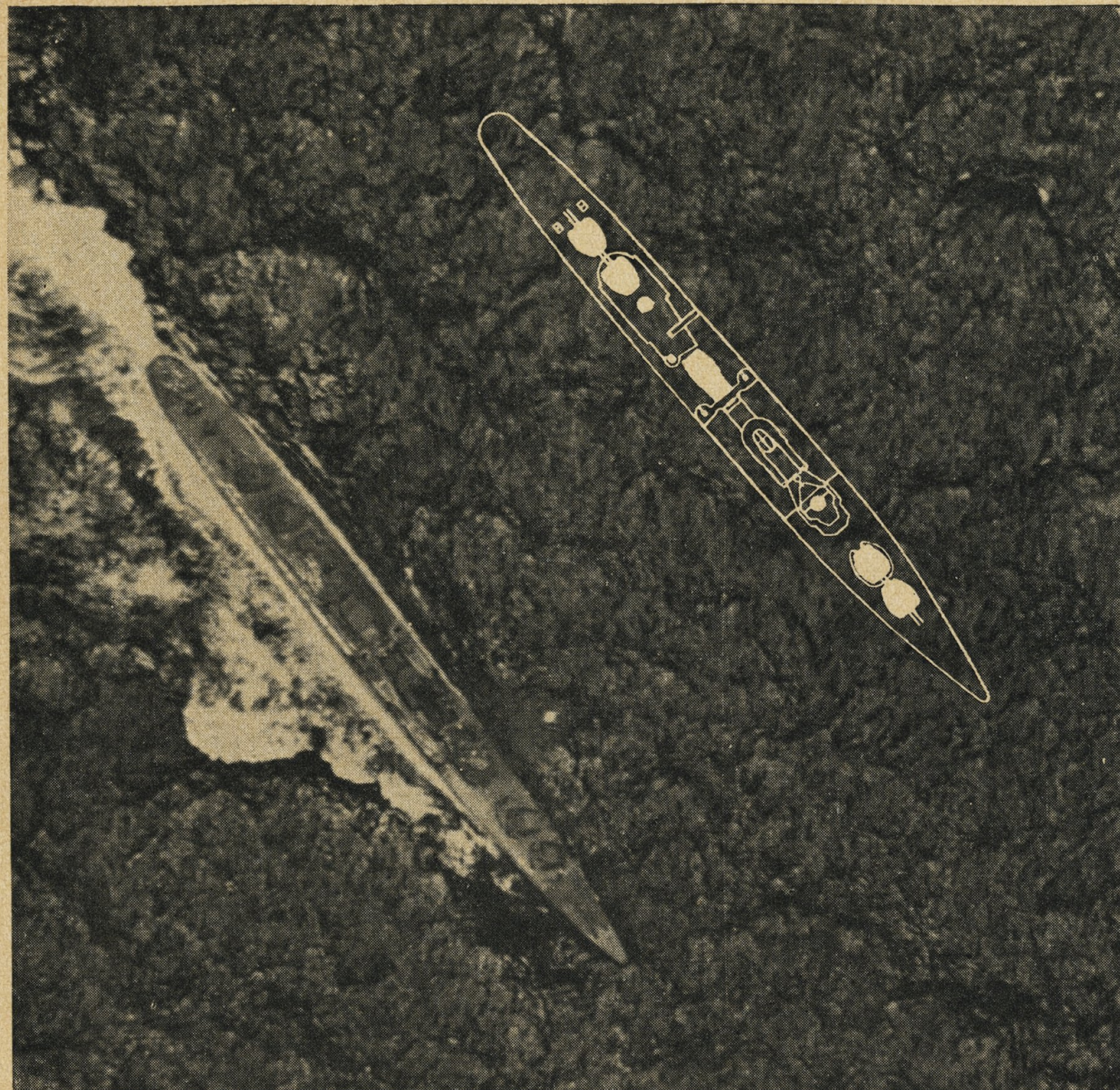
One of the new class of large Japanese destroyers, tentatively called TERATSUKI. A radical departure from previous Japanese ships of this type. Note the single raked stack and new type of "turtle-back" twin mounts.
