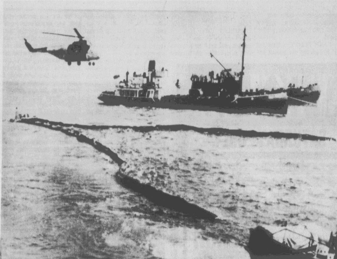
SKIMMER FOR OIL SPILLAGES — Tugboats tow a twin-hulled skimmer and booms during a demonstration off Portsmouth, England of an oil recovery system, called Oleanic. The procedure, developed at the Portsmouth Naval Base, is said to be able to deal with spillages in harbors and the hke. It is expected to recover 50 tons of oil an hour. (AP Wirephoto)
