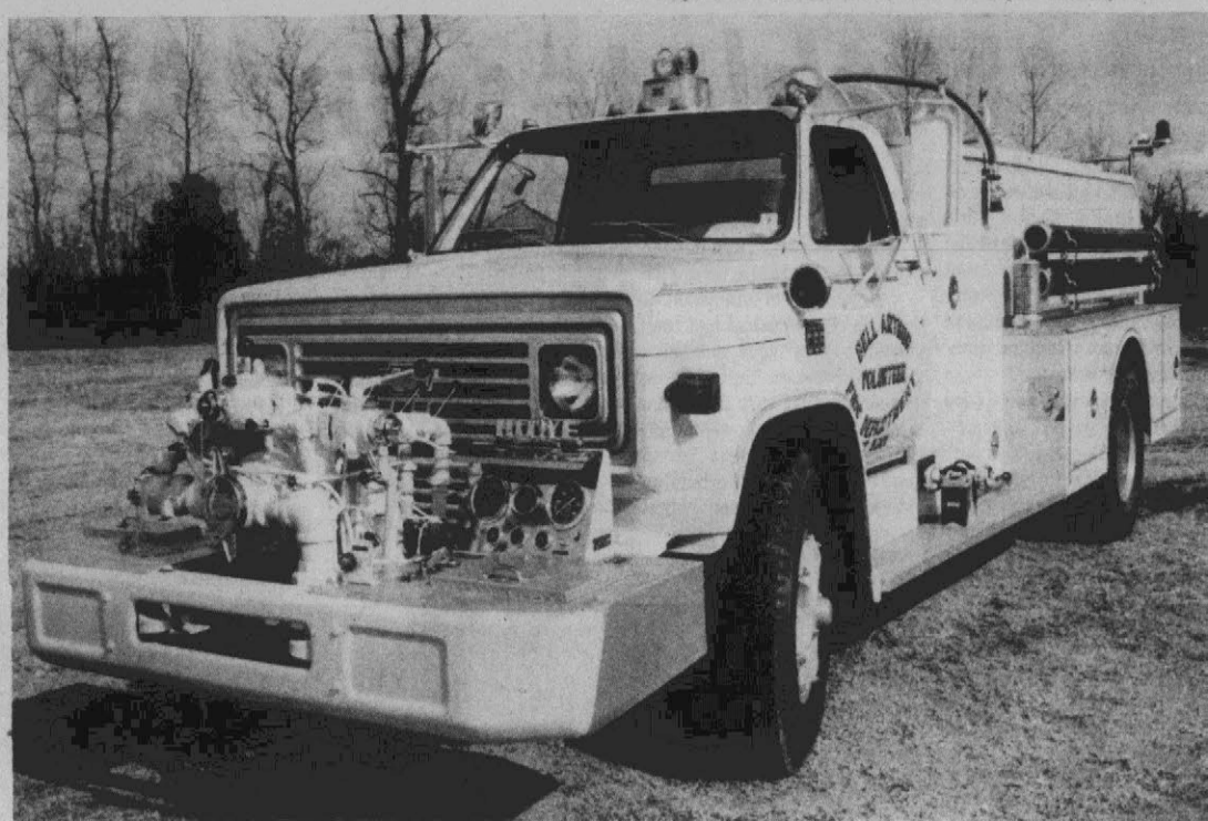
NEW FIRE TRUCK —The Bell Arthur Fire department recently purchased a new fire truck. The pumper is capable of pumping 750 gallons a minute and carrying 1000 gallons of water. Costing approximately $33,000, the new unit will be an addition to the existing two trucks now in service. (Reflector Photo by Tommy Forrest)
