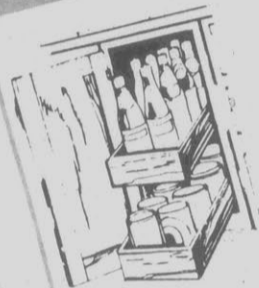
Roll Out Drawers Easy to reach, good for access to pots and pans, up to 36" wide.
