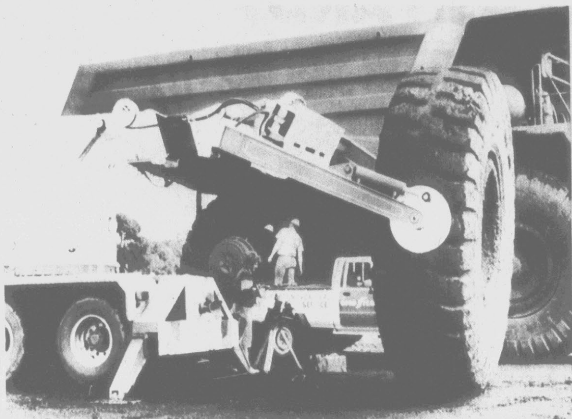
TIRE CHANGE? — A Goodyear earthmover tire is moved into position by a truck-mounted tire handler at a mine site in Muswellbrook, New South Wales, Australia.
