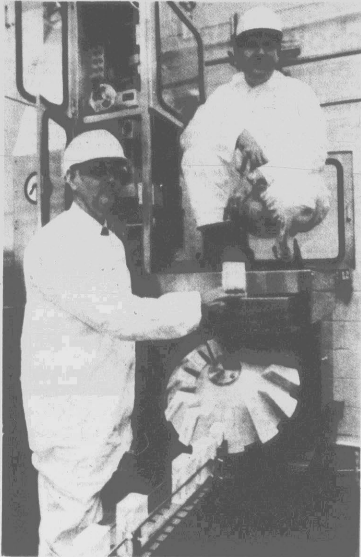
NEW PROCESS — N.C. State University scientists Dr. Hersell R. Ball Jr., left, and Dr. Kenneth R. Swartzel demonstrate equipment for aseptic packaging of fluid eggs. The equipment is part of a new process developed at NCSU to give eggs a longer shelf life without freezing. (AP Laserphoto)
