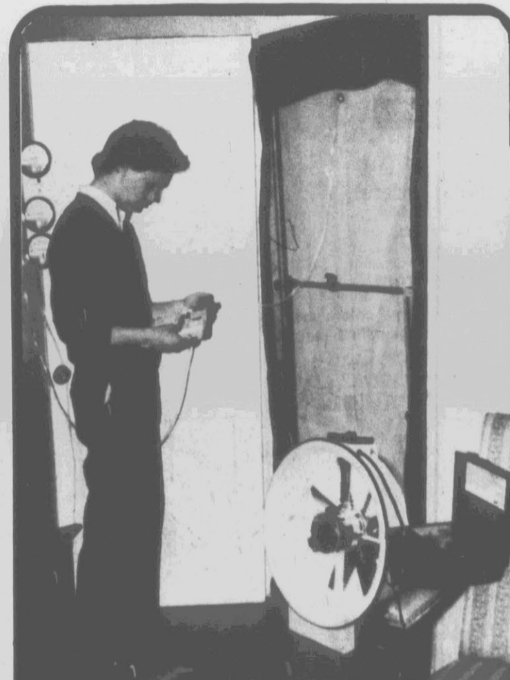
Energy Services Officer, Scott Jones, operates Greenville Utilities' portable blower door, a device used to locate leaks in homes.
