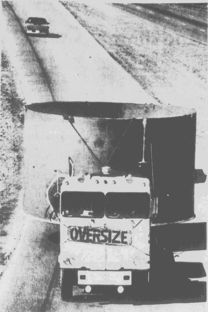
NO PASSING — A truck hauls the first section of a chemical storage tank to Bowater Carolina Co. near Rock Hill, S.C., blocking both lanes of traffic on one side of a divided highway. The section above was 18 feet in diameter and 10 feet high. (AP Laserphoto)
