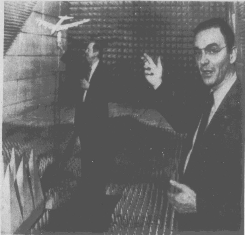
DEVELOPING 3-D RADAR — Dr. Joseph Bordogna, right, dean of the University of Pennsylvania's engineering school in Philadelphia, describes this echo-proof room being used at the school to develop a three-dimensional imaging radar system mimicking the way bats and dolphins bounce
