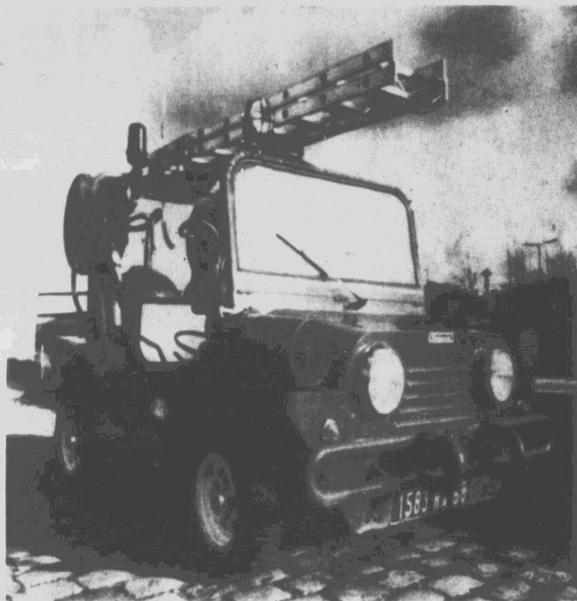
SMALLEST FIRE ENGINE — Produced by a French society of Saint Maur, Suburban Paris, the "MICRO 100" is powered by a British Leyland engine and is 2.35 meters long for 1.48 meters wide. Particularly adapted to urban areas, this vehicle is the world's smallest fire engine. (AP Laserphoto)
