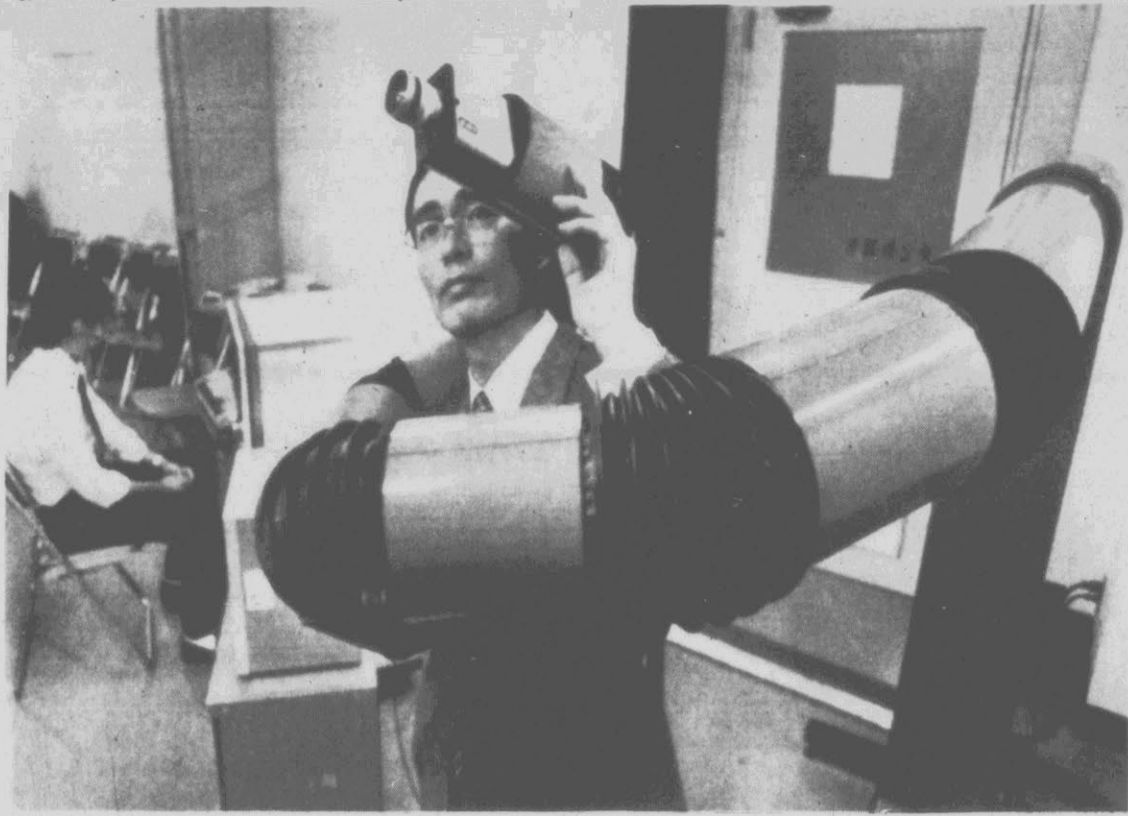
WRAPPED UP IN HIS WORK — Inventor Kuniji Asaho shows off a snake-like eight-jointed arm of an "inspection robot" he designed for Toshiba Corp. at its Kawasaki plant near Tokyo. The robot's TV camera-mounted arm can
