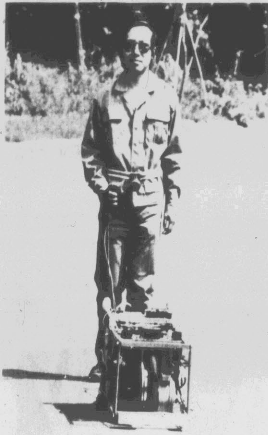
SEEING-EYE ROBOT — A researcher in Tokyo demonstrates MELDOG, a device built by scientists at the Ministry of International Trade and Industry to explore the concept of a mechanical seeing-eye dog for the blind. The developmental robot uses a variety of sensors to guide the blind "master" and warn of obstacles. (AP Laserphoto)
