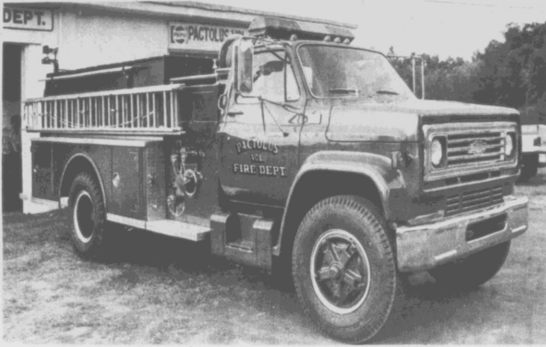
NEW PUMPER FOR FACTOLUS — The Pactolus Volunteer Fire Department took delivery last night of a new 1,000 gallon-per-minute pumper truck. The new unit was built by Atlas Steel of Raleigh, and was financed with an FHA loan of
