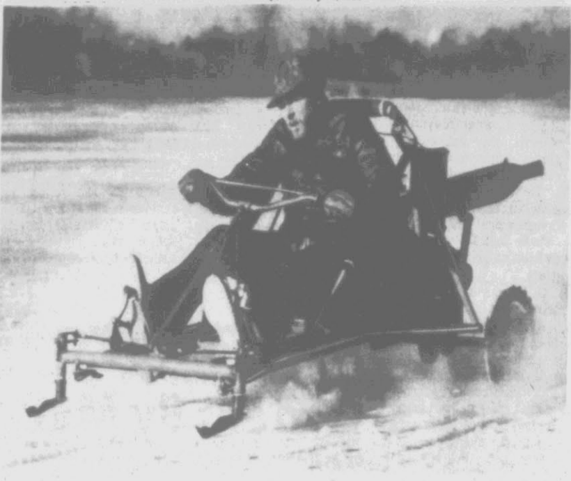
DO-IT-YOURSELF MOBILE — Joe Tupy, of Owatonna, Minn., enjoys a winter spin on the ice of Lake Kohlmer utilizing a motorcycle engine fitted to a handmade frame. It plys the surface of area lakes at speeds approaching 60 miles per hour, and was built from parts which cost about $75, excluding the engine. (AP Laserphoto)
