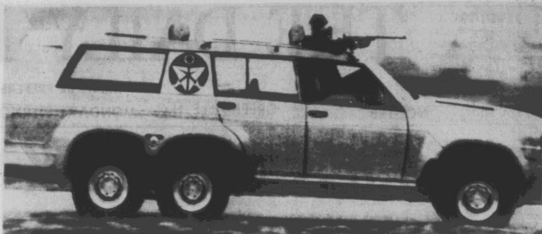
HUNTING CAR FOR SAUDI KING — The hunter's seat on this specially designed car can be raised 31.5 inches, giving the hunter a good shooting position. The six-wheeled car was built, as ordered, by Swiss designer Franco Sbarro for Saudi Arabian
