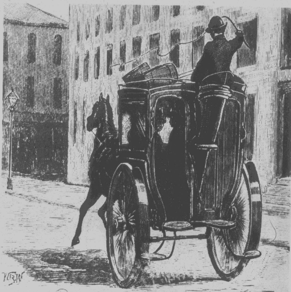
"Parlor" hansom of 1887 — a variation with seats for four passengers, entrance at rear.
