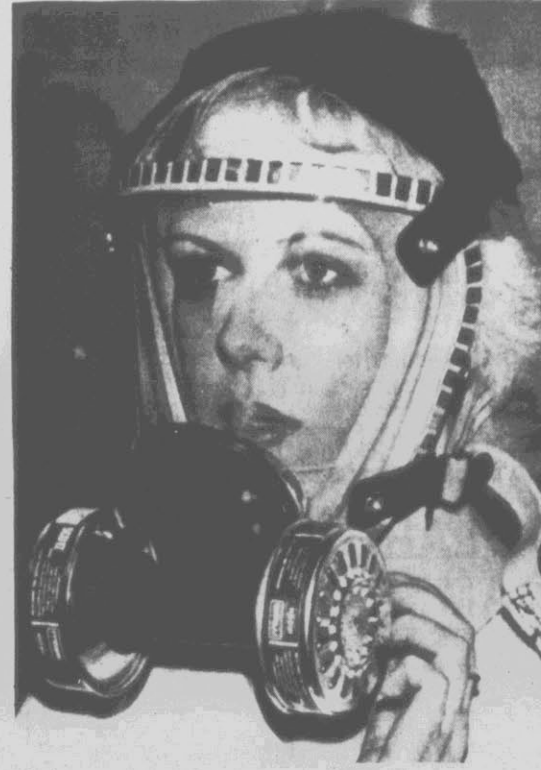
FLY ME TO THE MOON - Margaret Liszewski, engineering department employee at A-T-C Inc.'s Scott Aviation division in Lancaster, N.Y., tests a new face mask designed for female astronauts who are likely to be crew members on NASA's space shuttle. Because women's faces are generally rounder and smaller than men's, certain design changes in the men's masks are required. (AP Laserphoto)
