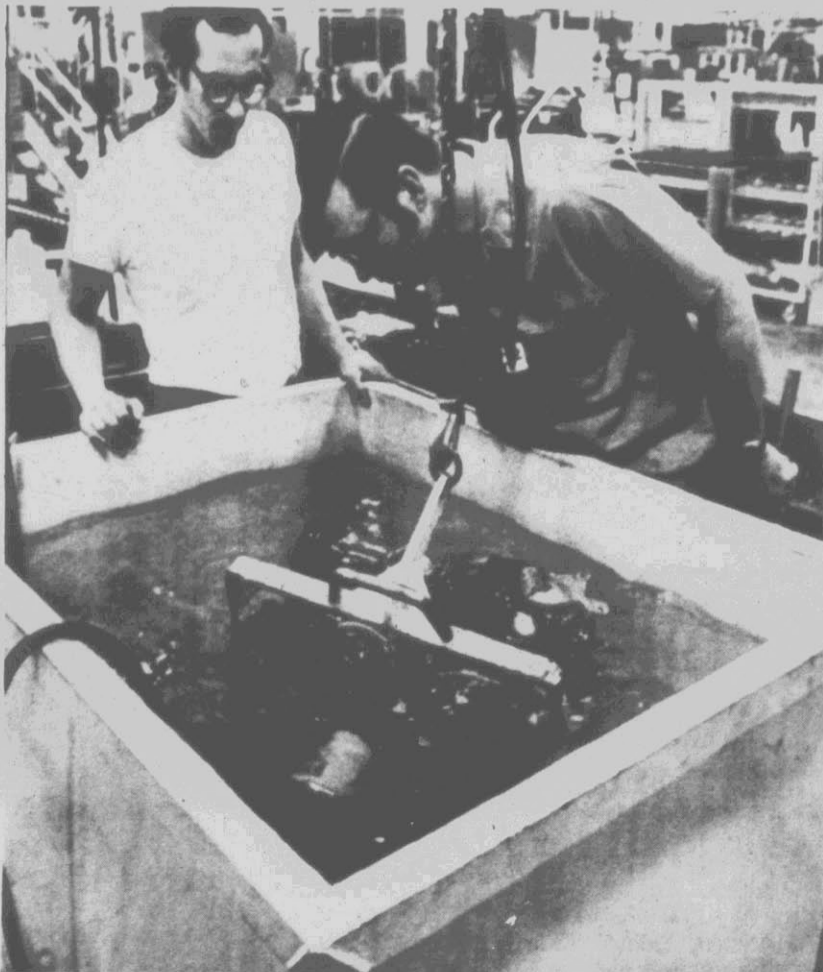
GETTING THE DUNK TEST — Workers at Chrysler Corporation's engine plant in Trenton, Mich., check out the four-cylinder engine which the automaker will use to power the 1981 K-cars. The suburban Detroit plant has
