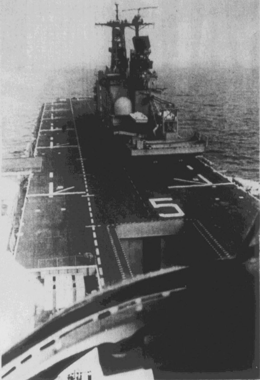
NEW ASSAULT SHIP — A helicopter approaches the flight deck of LHA-5, Peleliu, during sea trials in the Gulf of Mexico. The Peleliu is the fifth of the 820-foot-long amphibious assault ships built for the U.S. Navy by Litton Industries' Ingalls Shipbuilding division. The new 40,000-ton ship will be commis-
