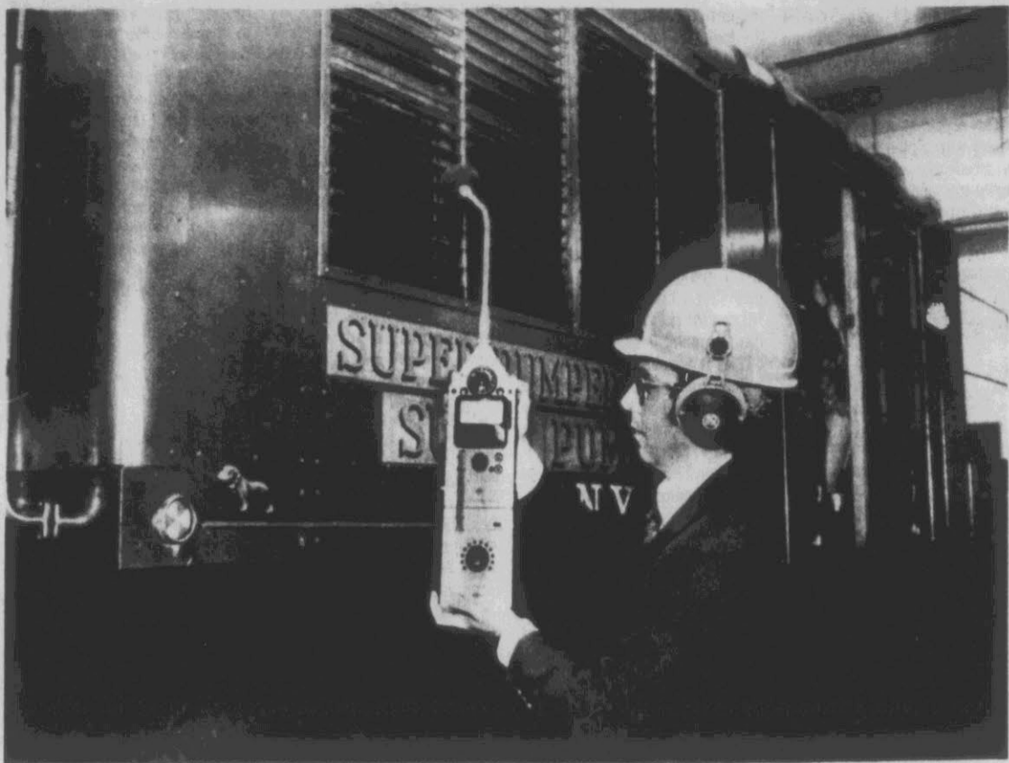
NOISES SCREENED — Dr. Marc Kramer holds a precision sound level meter near N.Y.C. Fire Dept. superpumper that knocks out walks with a stream of
