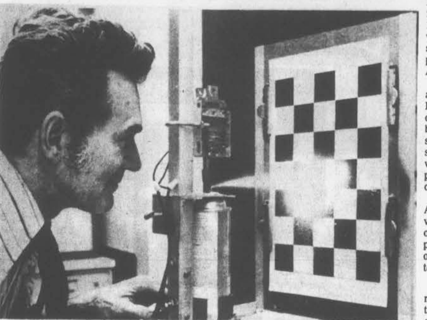
TESTING — This machine utilizes gameboard-like targets to test the spread pattern and covering power of spray paints. The one-of-a-kind device, designed by technicians at Woolworth's Quality Assurance Laboratory in New York, electronically triggers the spray for a controlled amount of time. Data obtained from the paint covered targets are used to evaluate products being considered for sale...or for monitoring the quality of products already on the shelf. (AP Laserphoto)
