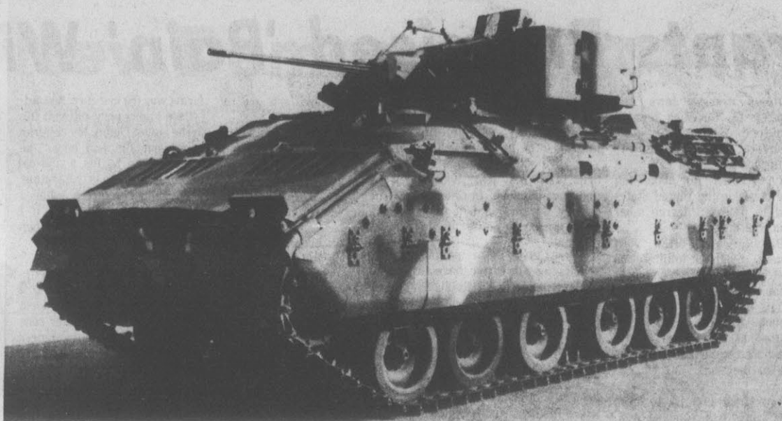
XM2 PROTOTYPE — The U.S. Army has taken delivery of the first two prototype XM2 Infantry Fighting Vehicles at the FMC Corp. plant in San Jose, Calif. An $80 million contract provides for eight test vehicles leading to production in 1981 if approved by Congress. Features include a 500 horsepower turbocharged diesel engine with automatic transmission and a top speed for 42 mph. A two-man turret with 25 mm automatic cannon, TOW missile anti-tank launcher and 7.62mm machine gun with six individual gunports. The new system weighs 47,000 pounds with combat load. Another version, the Cavalry Fighting Vehicle is called XM3. (AP Laserphoto)
