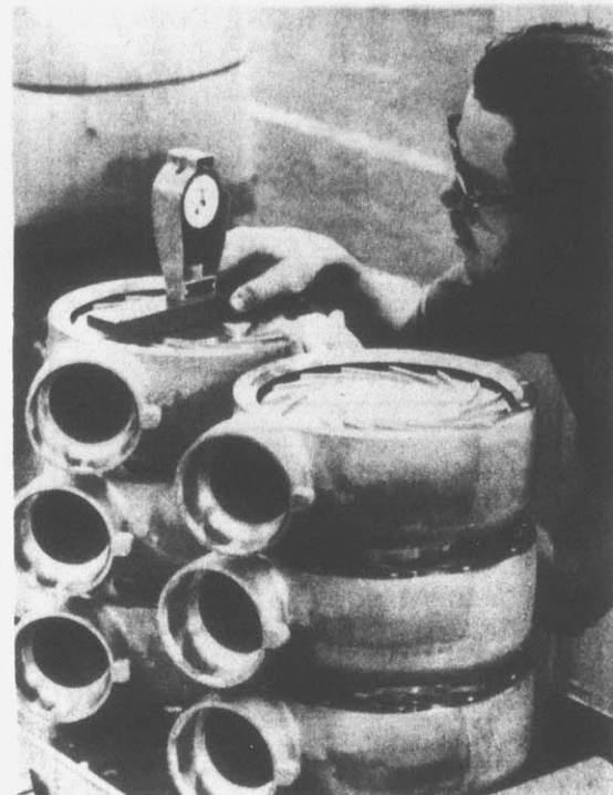
LITTLE BIT MEANS A LOT — Employee Leo Blankenship checks tolerances of turbochargers being made at Torrance, Calif. plant of Garrett Corp., one of the Signal Companies. If the tolerance varies more than two-thousandths of an inch, the turbocharger, used to boost power output of engines, will not work. (AP Laserphoto)
