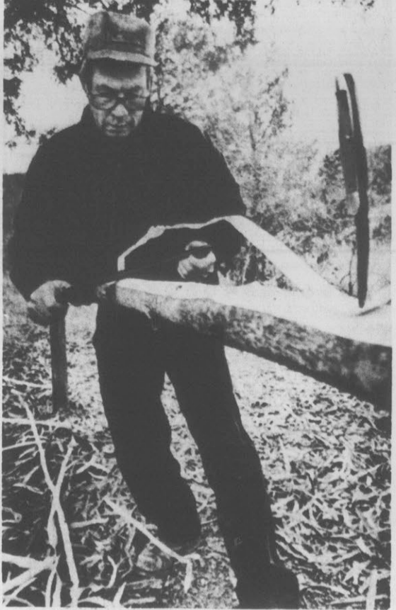
HICKORY STRIPS — Ozark mountain chairmaker Jack McCutcheon cuts a strip of the inner bark of the bitternut hickory tree after peeling off the outer bark with a draw knife. (AP Laserphoto)
