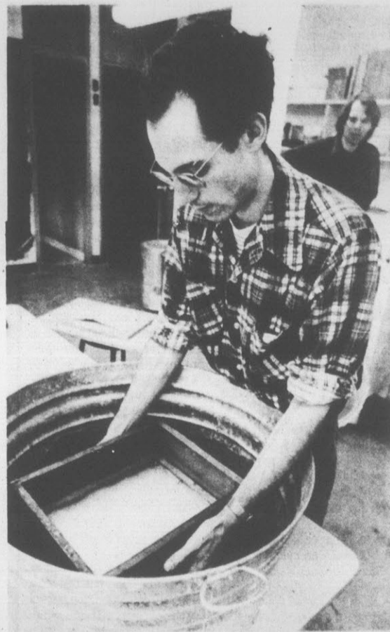
MOLDING THE PAPER — Ben Tauber shows how the paper is hand molded. The mold is dipped into a vat containing the pulp, shaken to cross the fibers, and the water drained out. (AP Laserphoto)
