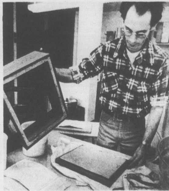
UNMOLDING THE PAPER — The thin, very wet piece of paper is released from the mold by Tauber. The paper is then placed on cotton material or blotters and the water is pressed out, which also compresses the fibers. (AP Laserphoto)
