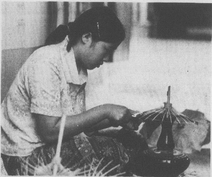
Paper cover is pasted on frame of miniature umbrella.
