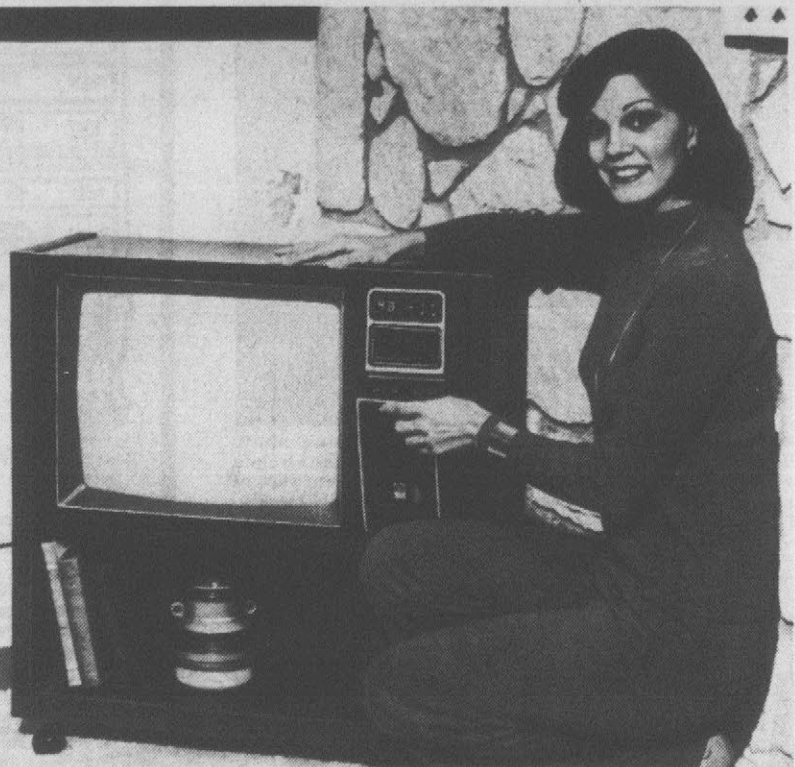
CONTEMPORARY STYLING/CONTEMPORARY ELECTRONICS — both here in General Electric's new 19-inch remote control, VIR "broadcast-controlled" color television. The set features full-remote controlled operation and VIR "broadcast-controlled" color adjustment. Through the use of a light dependent resistor system, contrast, brightness and color intensity are set according to room lighting conditions. The cabinet is styled with a walnut finish on high impact plastic with the designed coordinated base offered as an optional extra.
