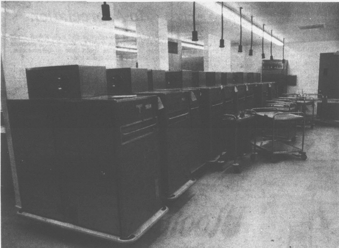
DIETARY UNITS... Carrying units for food to patient floors are in the kitchen area of the new facility. The units have a hot and cold section and can be plugged in on each floor.
