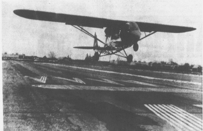
BREEZY IN FLIGHT — Pilot Gil Baker, 56, takes off from Big Beaver Airport aboard "Breezy," an experimental aircraft built by members of the Detroit Chapter, Experimental Aircraft Association. The steel-tubed monoplane is powered by a 125-horsepower engine which reaches a maximum speed of 75 m.p.h. The plane was built to celebrate the 73rd anniversary of Orville Wright's landmark flight. (AP Wirephoto)
