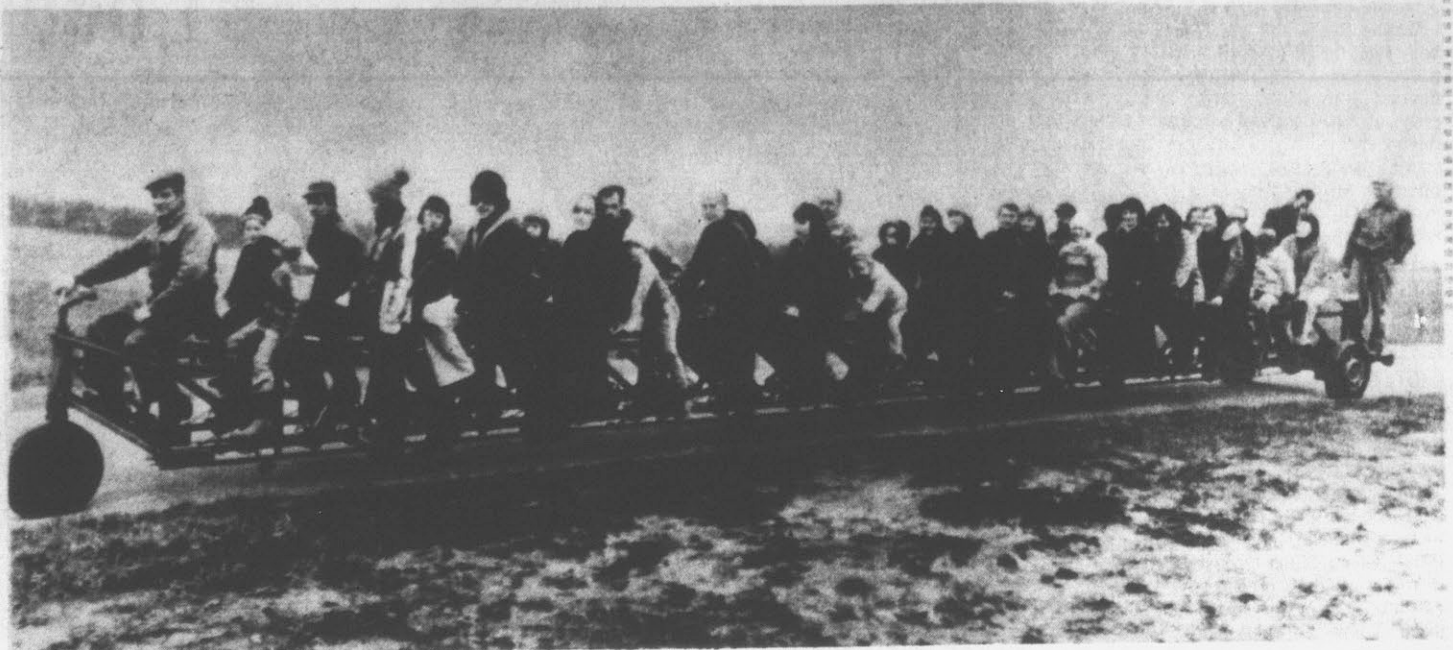
A BICYCLE BUILT FOR 35 — Hop on this bicycle built for 35 made from 78 old cycles, 70 sprocket wheels, 165 feet of chain, 130 steam pipes and three car wheels. On their first try the daring group pedaled several hundred feet in Hadsund, Jutland, where the bike was put together. (AP Wirephoto)
