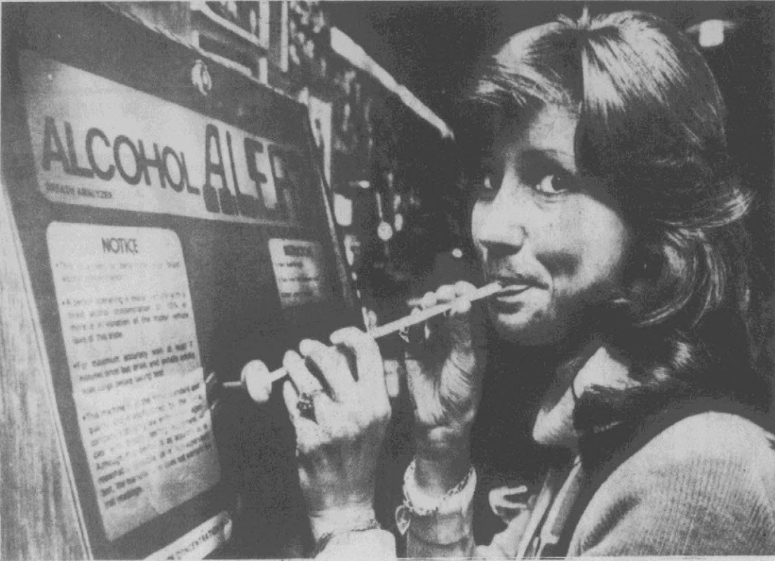
TESTING — Maria McBane blows a sample of her breath into a machine called "Alcohol Alert" in Los Angeles. The machine, after the user deposits a quarter, according to the developer of the device, could be used in bars to let drinkers know when they've had too much to drive. The developer says the machine is as accurate a device as any used by the police department. (AP Wirephoto)
