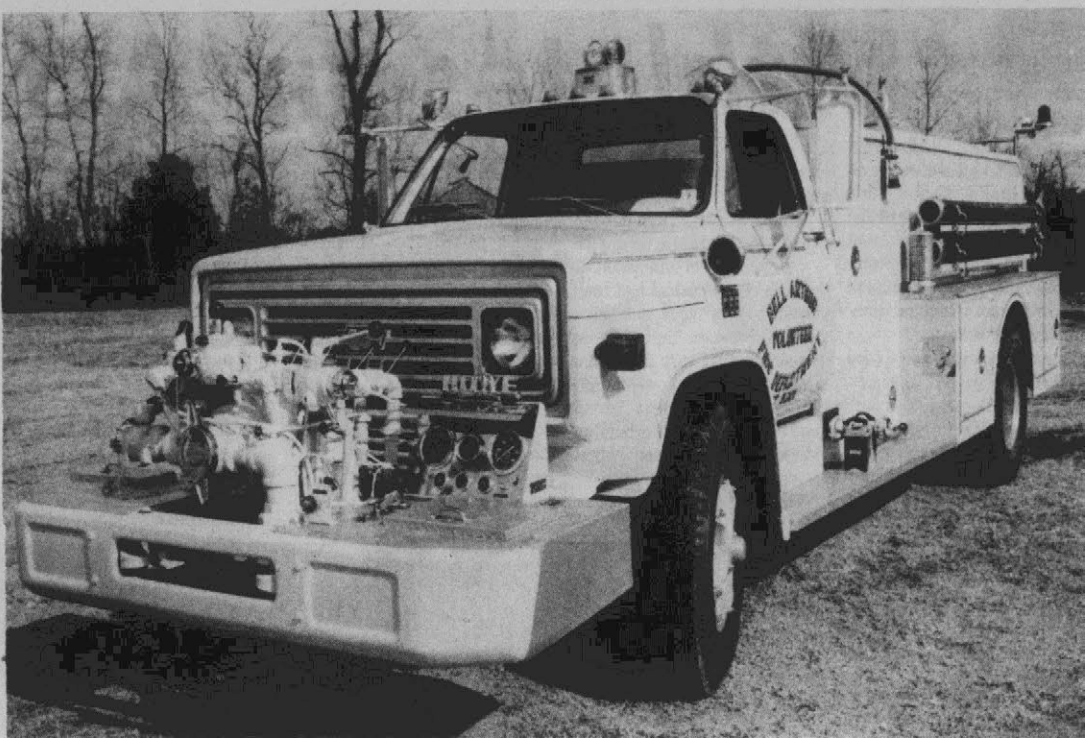
NEW FIRE TRUCK —The Bell Arthur Fire department recently purchased a new fire truck. The pumper is capable of pumping 750 gallons a minute and carrying 1000 gallons of water. Costing ap-
