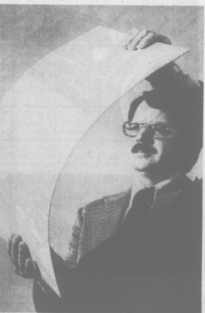
FLEXIBLE CEMENT—A panel of flexible cement reinforced with fiber glass is shown to have certain properties approaching those of reinforced plastics. Such high-strength, fireproof panels are being developed by the Fiber Glass Division of PPG Industries. The glass-reinforced cement products are made from readily available inorganic materials. (AP Wirephoto)
