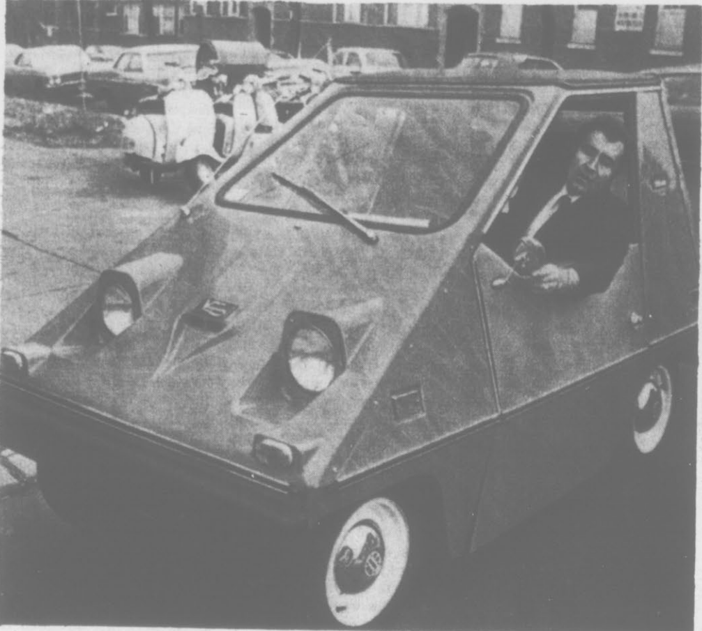
ON THE MOVE—Chicago auto dealer Guy Beaufort checks for traffic before pulling out in his Vanguard electric car at Chicago. Beaufort says sales of the 1100-pound, 2½ horsepower auto are increasing. It is believed to be the cheapest American-made car, listing for $2,390. It has maximum speed of 28 miles an hour and can be recharged overnight in any 110-volt household outlet for 18 cents. (AP Wirephoto)
