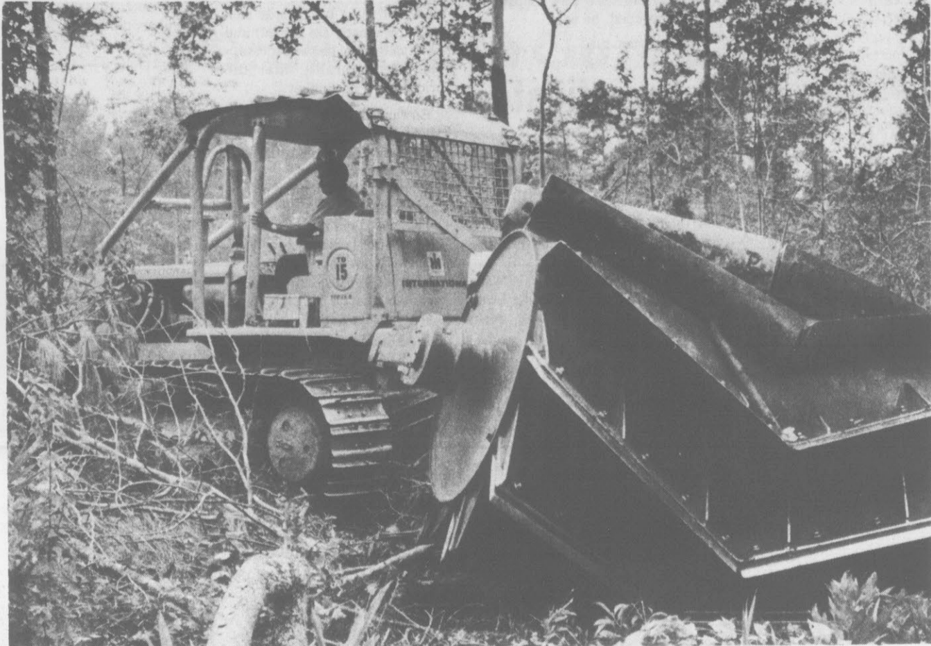
SITE PREPARATION WORK. Site preparation work is being done by a private contractor this summer so that loblolly pines can be planted on this land next spring. A drum chopper is used to clear the
