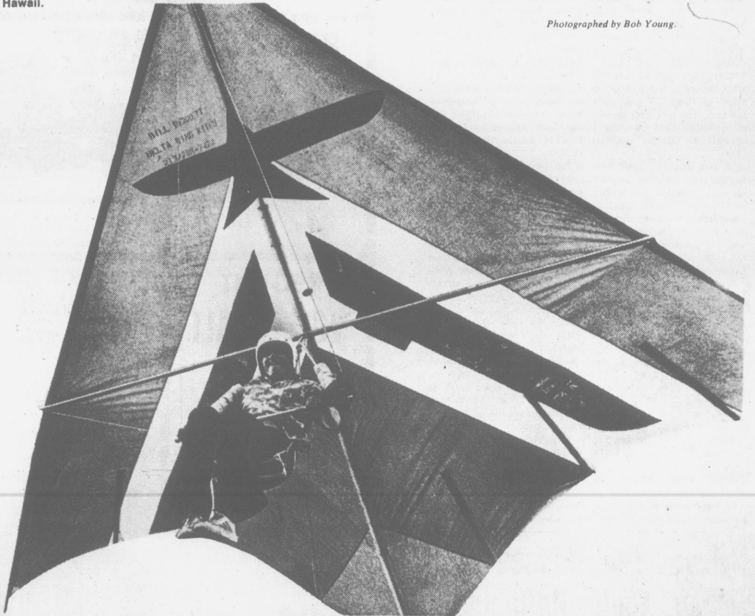
Basic shape of hang-gliders is the Rogallo wing, developed by NASA scientist Francis Rogallo.
