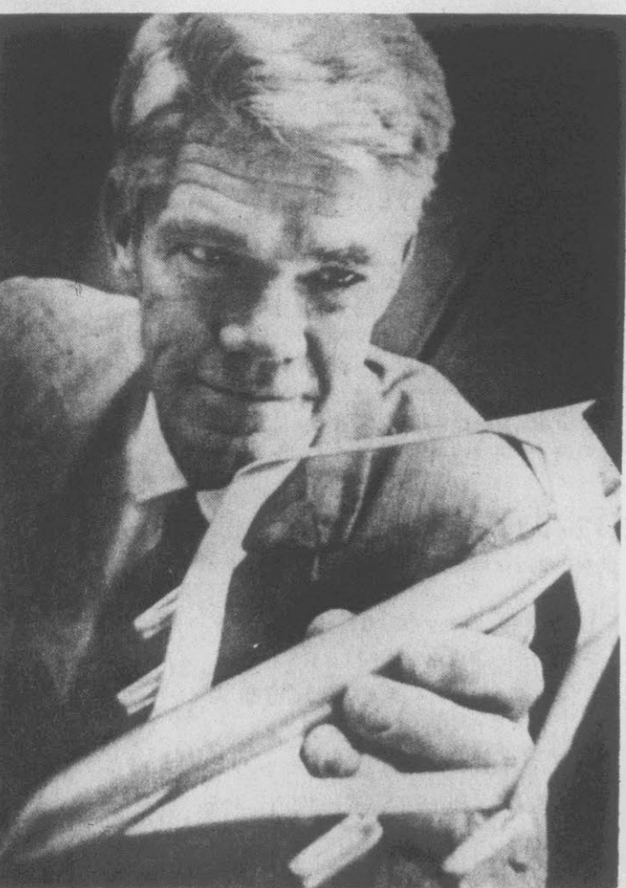
REVOLUTIONARY DESIGN — Jones F. Cahill, an aeronautical engineer with the Lockheed-Georgia Company at Marietta, displays a model of a passenger biplane that he has designed. The almost hexagon-shaped biplane has a forward wing which sweeps backward and a rear wing which sweeps forward, joined together at the wing tip by vertical fins. The 400-passenger plane would cruise just below the speed of sound—or about 630 miles per hour. (AP Wirephoto)
