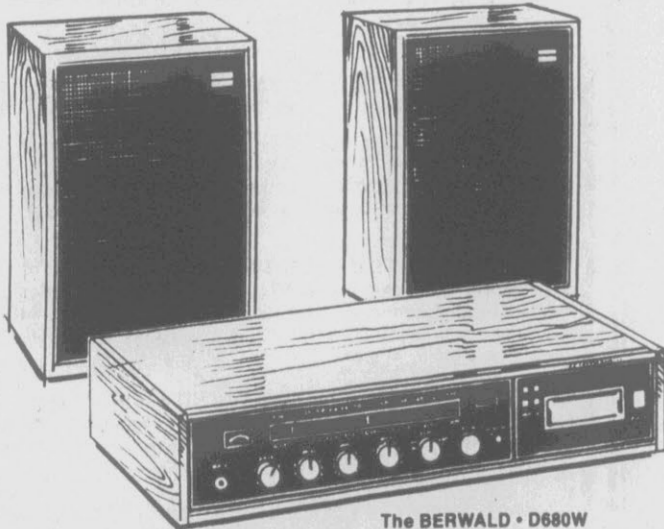
The BERWALD • D680W Built-in 8-Track cartridge player. FM/AM/Stereo FM tuner/amp. 20 Watts of peak power output. Solid-state amplifier. Tuning meter. Stereo headphone jack. Each enclosure contains one 6 1/2" round woofer and one 2" tweeter. Cabinets in wood grained Walnut veneers.
