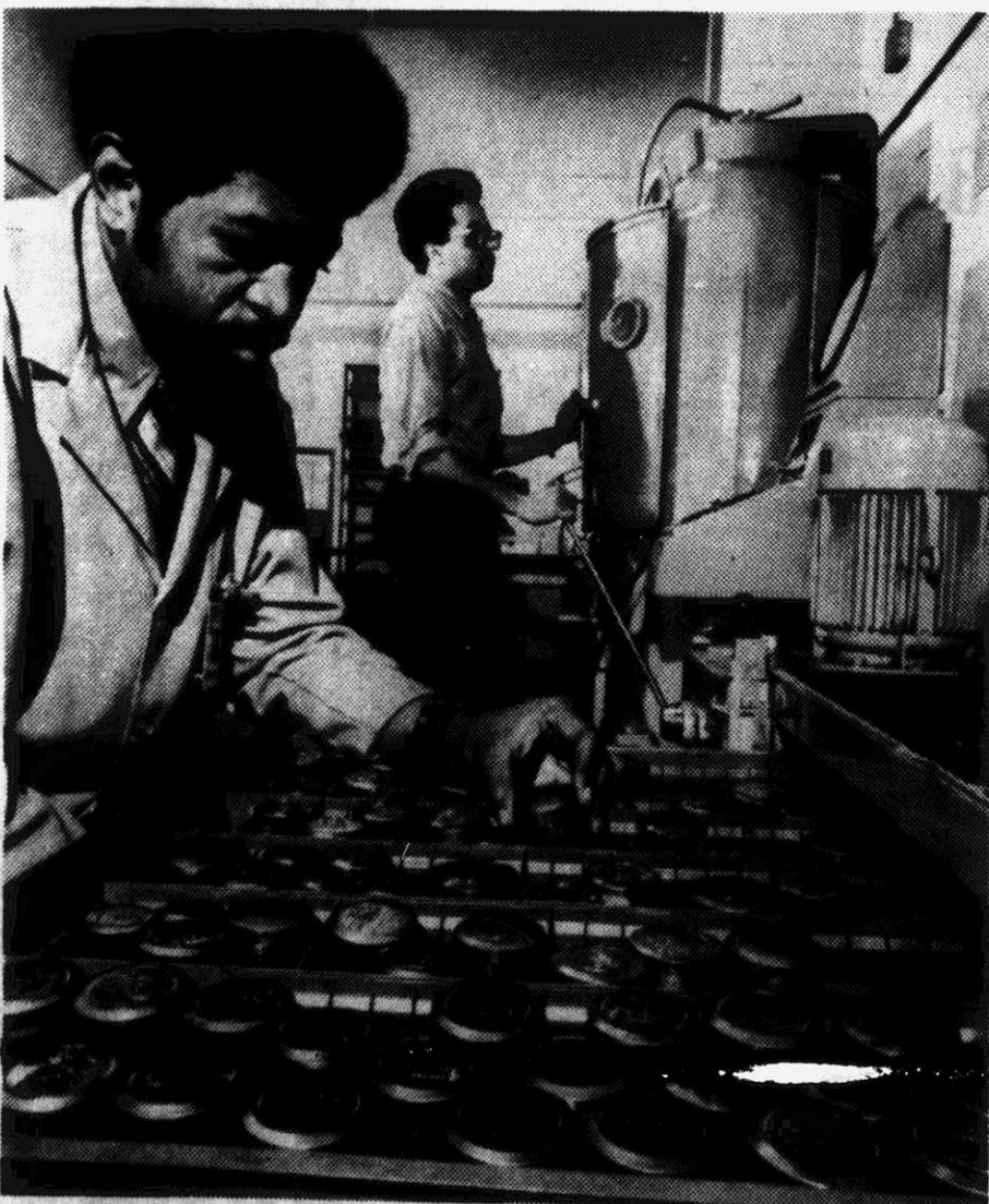
Master engraving is picked for die making in hydraulic press, rear.
