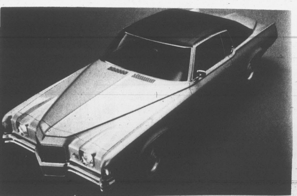
GRAND PRIX, 1971 — High-intensity single headlights, a new vertical bar grille and a two-level bumper highlight the front of the restyled 1971 Grand Prix. The rear has a classic boat tail with new quarter panels, deck lid, bumper and taillights. Standard equipment includes variable ratio power steering, power front disc brakes and a 400 cubic-inch V-8 engine. The SJ package includes a 455 cubic-inch power plant.
