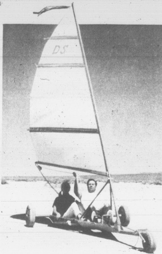
Three-wheeled "boat" can whip along at up to 50 mph, is steered by pedals up front.
