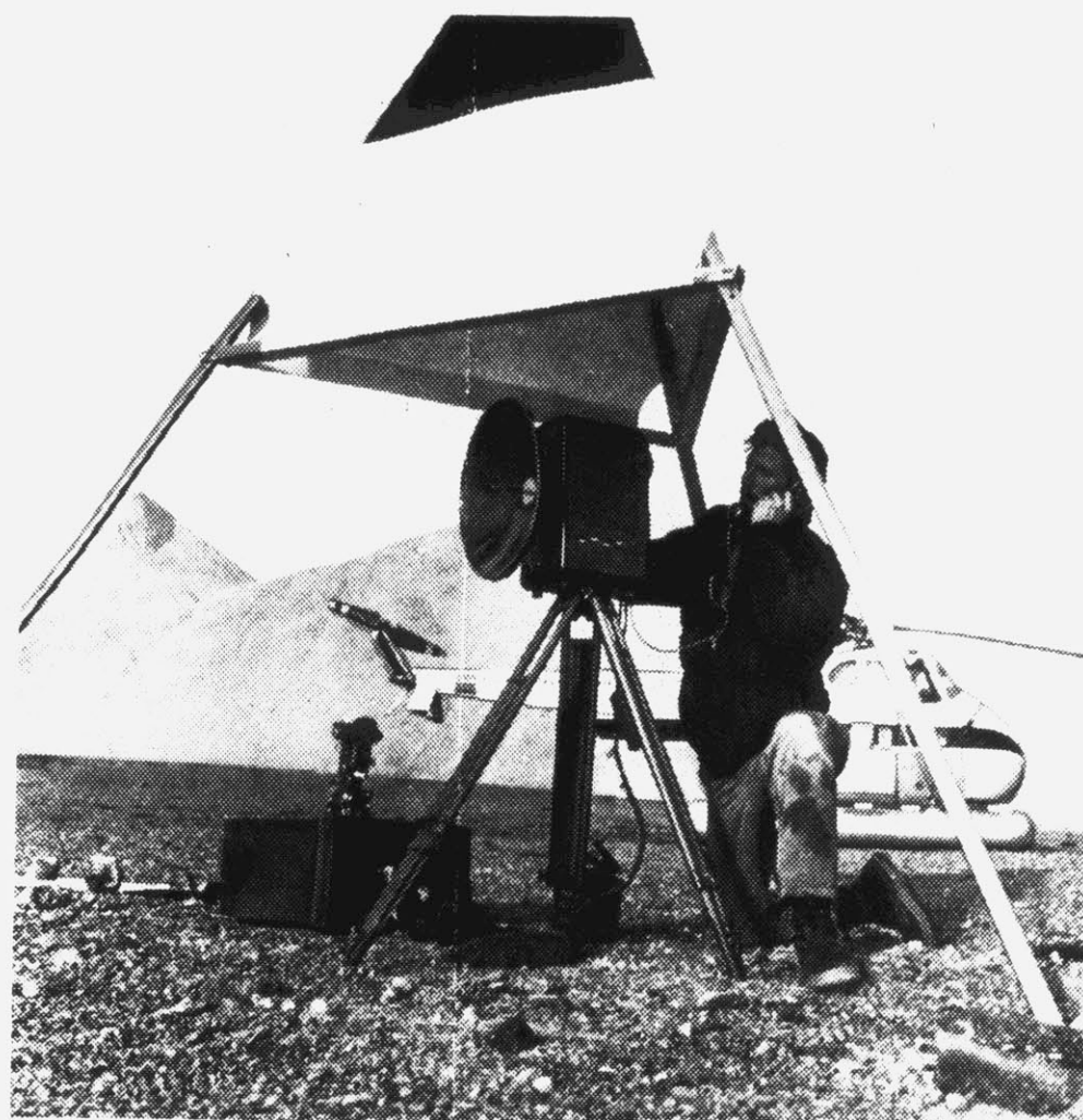
Topographical surveyor uses tellurometer (electronic distance measurer) on arctic island.
