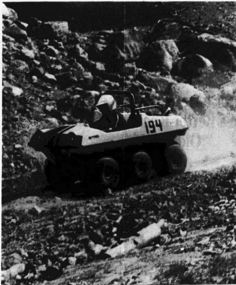
ROLL BARS are protection should the vehicle turn over on the rough race course.
