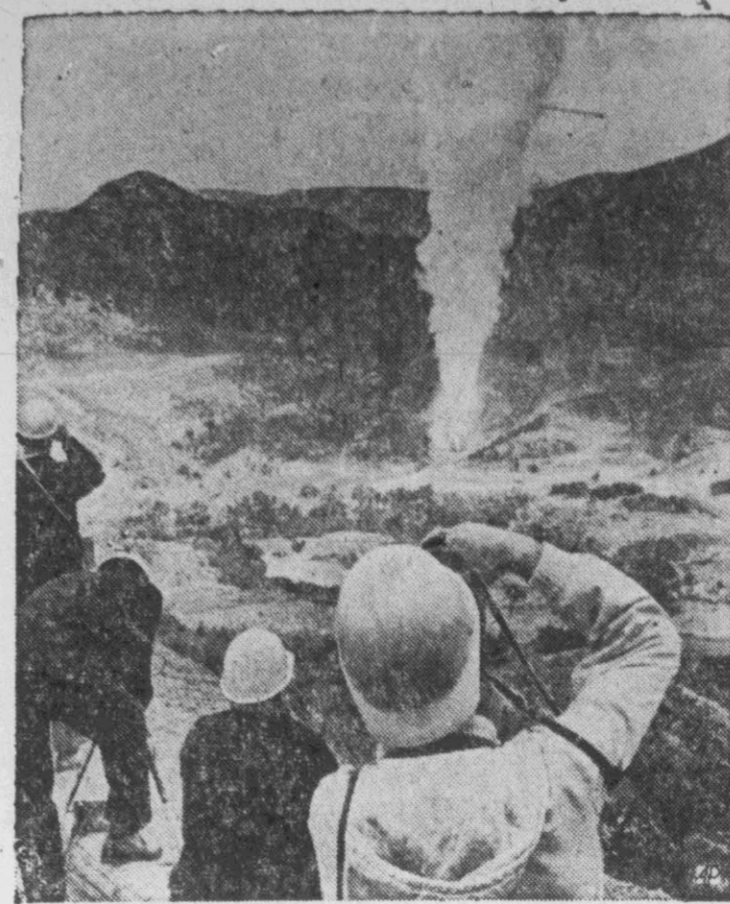
ROCKET TEST —Flame and smoke spurt from new solid-fuel rocket motor during test at Redlands, Calif. Manufacturer said it produced thrust of 400,000 pounds.
